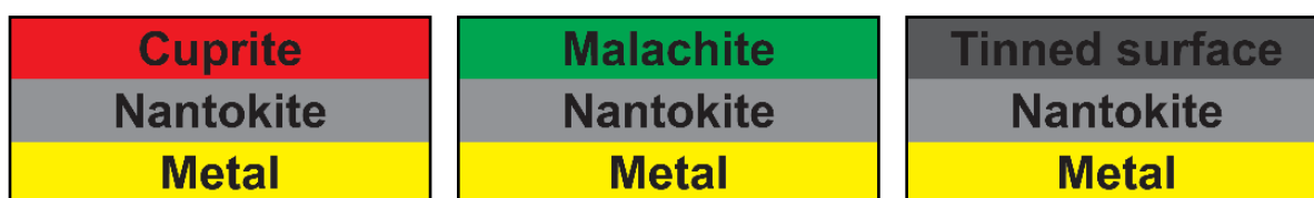
Figure 1 Schéma des systèmes de corrosion nantokite-cuprite (A), nantokite-cuprite-malachite (B), nantokite-étamage (C). © N. Gutknecht, He Arc, 2018.
